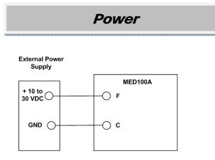
7. An external 10 to 30 VDC power supply is required. Attach power leads as shown above.
